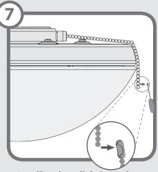
Installing the pull chain pendant Attach the pull chain pendant to the
